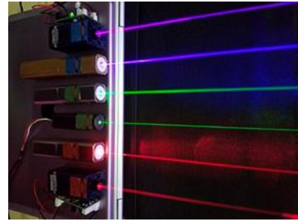
Red (660 & 635 nm), green (532 & 520 nm), and blue-violet (445 & 405 nm) lasers
